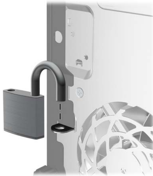
Figure 3-34 Installing a Padlock
